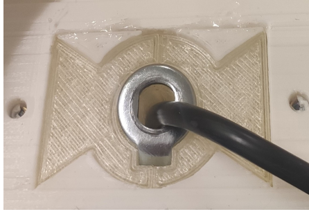
(a) Kite tail shaped element inserted in the robot's chassis.
